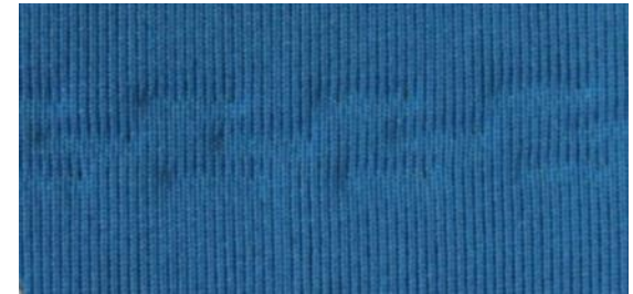
laser welded seam
