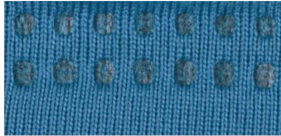
ultrasonic welded seam
