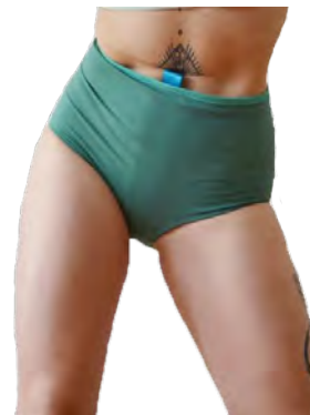
Textile-based soft biosensor integrated into underwear for detection of vaginal infections by Alma & IZM, © Giulia Tomasello
