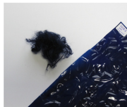
Lyocell-Composite-Material with 10 % Prussian Blue
