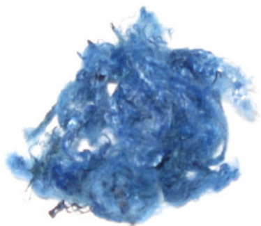
Cellulose fibres treated with chemicals to build Prussian blue in situ
